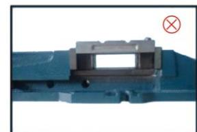
It is not easy to be clamped. For example, the aluminum sheet is easy to flatten. The area to be clamped should be a little more. Supported
