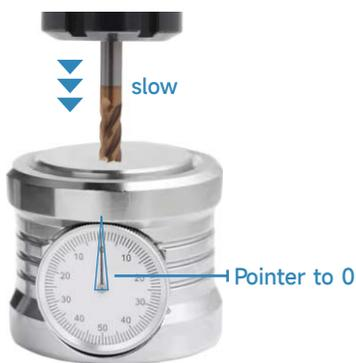
Rotate the dial indicator pointer to zero and start calibration
