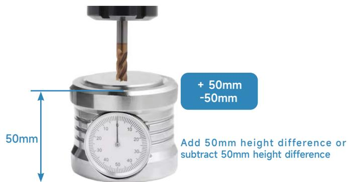
Put the Z-axis setter on the workpiece, and the tool contacts the measuring surface. Slowly feed the tool so that the pointer is at "0". The distance between the tool and the upper tool is equal, and the height difference distance between the tool and the workpiece is 50mm
