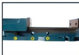
Remember the three small holes ABC, open each time increase by 100mm, aim at the inner tooth seat Otherwise you will get stuck
